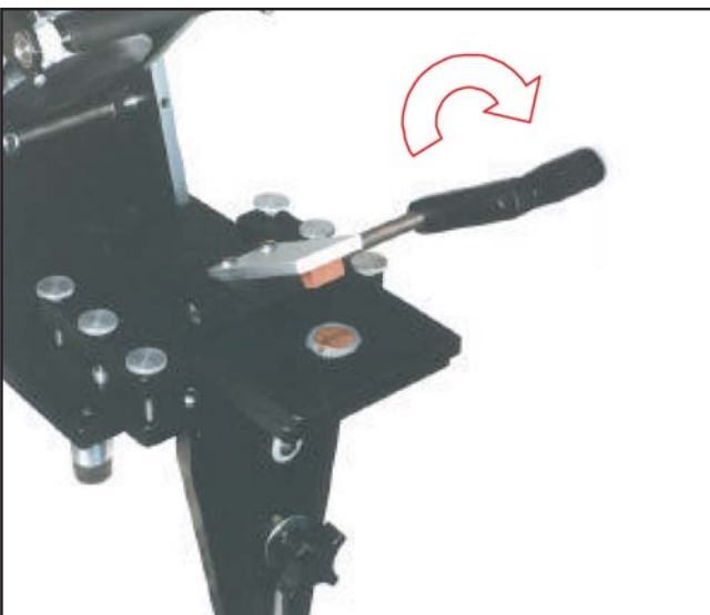
Precision placement fixture for 'hard to reach' surfaces such as depressions or close to obstructions
