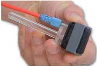
Clip the red lead to the marking head. The marking head holds a felt pad and a thin mesh which improves the print quality
