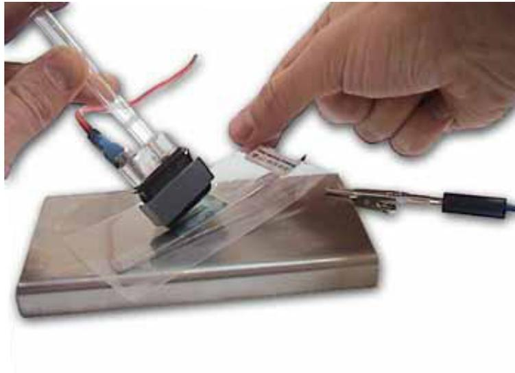
After marking is done, remove excess electrolyte from part
